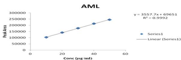
Fig. 5: Calibration curve of amlodipine besylate (AML)
