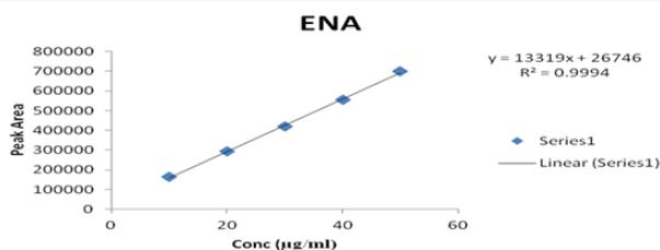
Fig. 6: Calibration curve of enalapril maleate (ENA)
