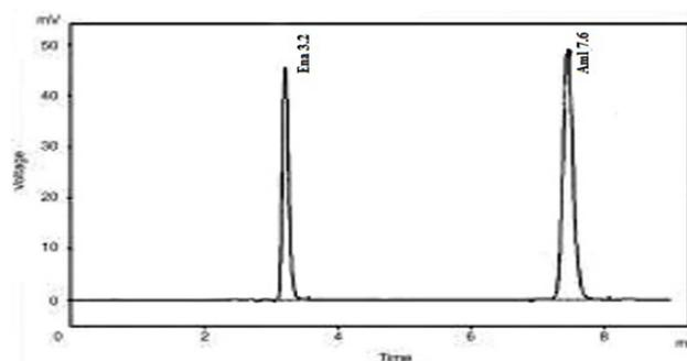
**Fig. 3:** Chromatogram Report of Amlodipine besylate & Enalapril maleate For Amlodipine besylate RT = 7.6 min For Enalapril maleate RT = 3.2 min
